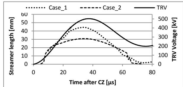
Fig.4: Evolution of streamer length for 245kV cases in parallel with the TRV evolution
