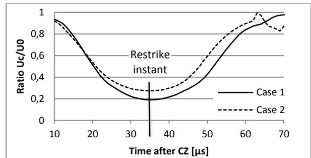
Fig.6: Criterion results in parallel with breakdown instant
