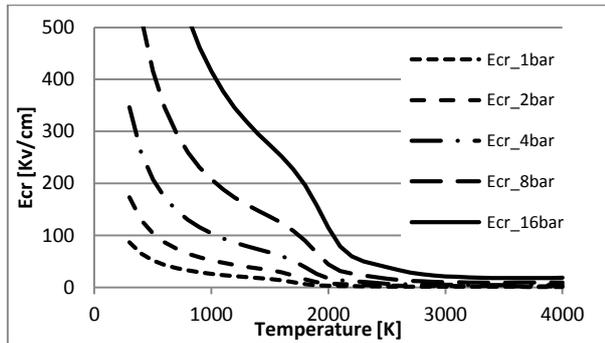
Fig.1: Evolution of the critical electric field for SF6 at several pressures
