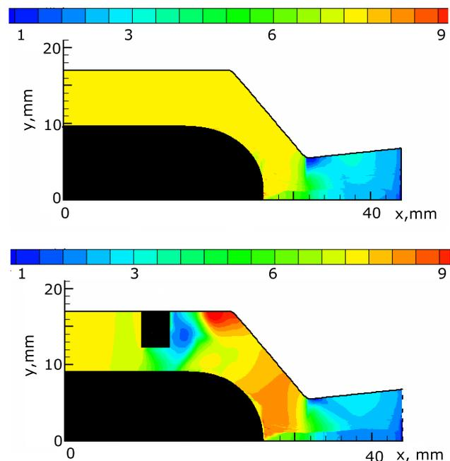
Fig.4: The pressure field in (a) the standard extinguishing chamber and (b) arc-extinguishing chamber equip with open heating volume of the section area ratio  $S/S^* = 2.5$
