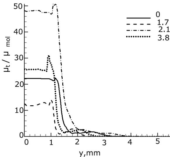
Fig.3: The turbulent and molecule viscosity ratio in the nozzle throat at different values of the section area ratios,  $S/S^*$
