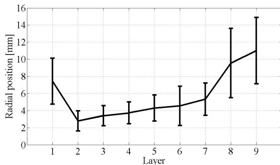
Fig. 6: Arc position for a time range of 40  $\mu$ s before current zero (cf. Fig. 1)
