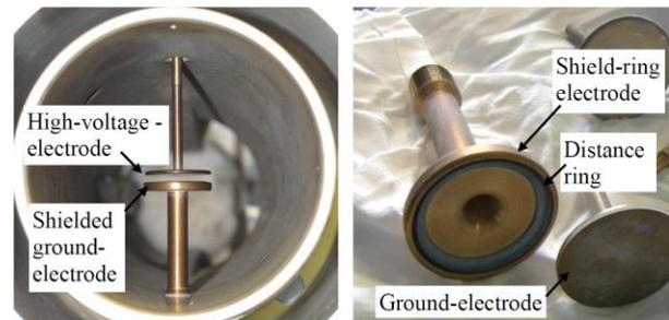
Fig.1: Sensor electrodes in the switching chamber
