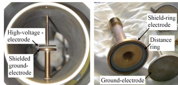
Fig.1: Sensor electrodes in the switching chamber
