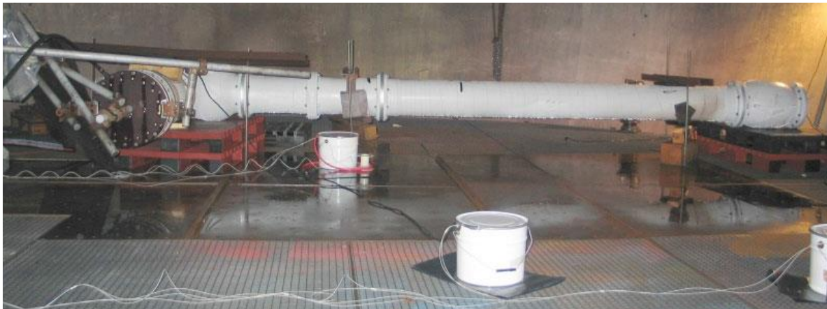
Fig.1: Picture of a long single phase HV-GIS. It is 5.5m long and has a diameter of 30 cm
