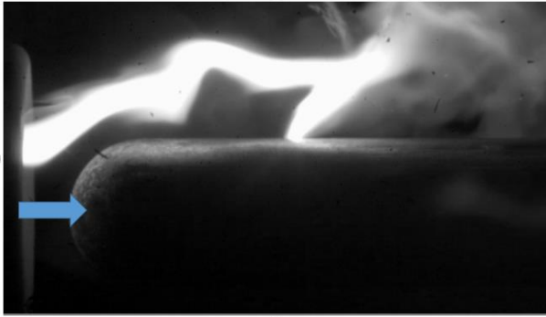
Fig. 7: Arc drifts away from the axis due to increased blowing; arrow shows the axis where maximum blowing occurs
