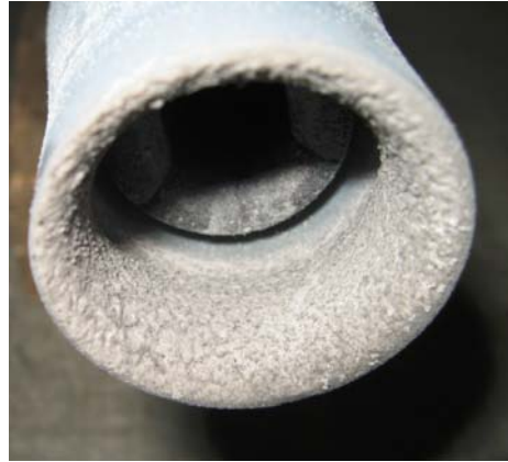
Fig. 4: PTFE nozzle after arcing
