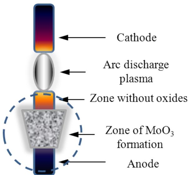
Figure 1. Electrodes arrangement for fabrication of  $\text{MoO}_3$  crystals
