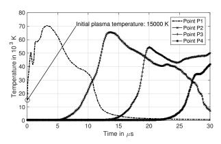
Figure 4. Temperature behaviour of the plasma in dependence of the time.
