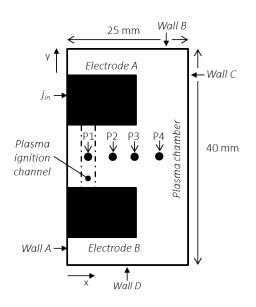
Figure 1. 2D geometry for which the computational model is solved
