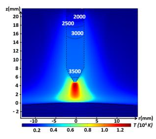
Figure 2. Two-dimensional distribution of the plasma temperature and the temperature in the electrodes obtained with the LTE model for an arc in  $CO_2$  at current of 200 A.
