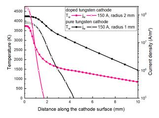
Figure 4. Temperature and normal current density along cathode surface for doped and pure tungsten cathodes for an arc current of 150 A.
