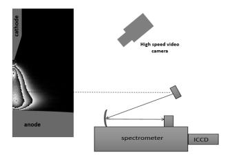
Figure 1. A view of the computational domain and the OES arrangement used for investigation of the arc.
