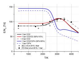
Figure 5. Predicted particle density reduced critical fields normalized to standard conditions of 300 K and 1 bar for  $CO_2/O_2$ ,  $CO_2$  and  $CO_2/O_2/C_2F_4$  mixtures. Literature values for  $CO_2$  are given by the symbols.
