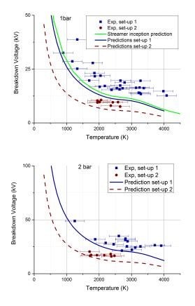
Figure 3. Breakdown voltages in  $CO_2/O_2$  mixture vs temperature at 1 and 2 bar.
