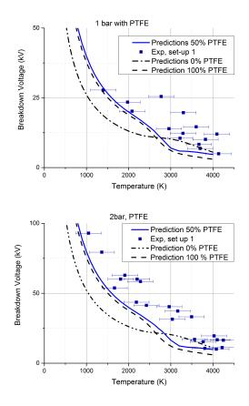
Figure 4. Breakdown voltages in  $CO_2/O_2/C_2F_4$  mixture vs temperature at 1 and 2 bar.
