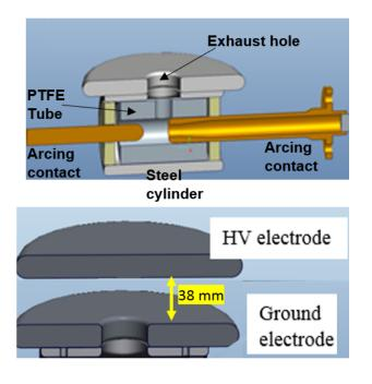
Figure 1. Hot gas generator and exhaust hole in ground electrode (top), electrode arrangement of set-up 1 (bot-tom).
