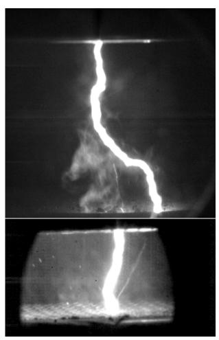
Figure 2. Breakdowns at 1 bar in set-up 1 (top) and set-up 2 (bottom).
