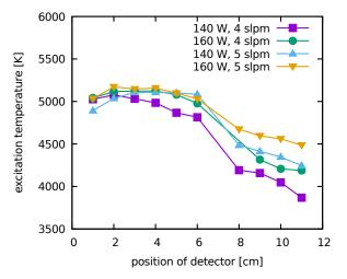
Figure 6. Excitation temperature profile from the argon lines without aerosol for different power and working gas flow rate.
