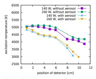
Figure 8. Excitation temperature profile from the argon lines with and without aerosol for different power for same working gas flow rate (4 slpm).
