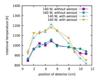
Figure 5. Rotational temperature profile along the discharge axis with and without aerosol for different power for same working gas flow rate (4 slpm).
