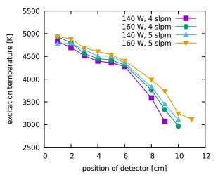
Figure 7. Excitation temperature profile from the argon lines with aerosol for different power and working gas flow rate.
