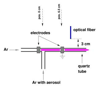
Figure 1. Experimental arrangement of the discharge.
