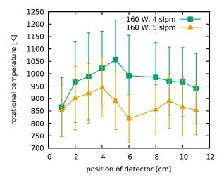
Figure 3. Rotational temperature profile along the discharge axis without aerosol for power 160 W and different working gas flow rate with error bars.
