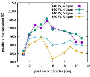
Figure 2. Rotational temperature profile along the discharge axis without aerosol for different power and working gas flow rate.
