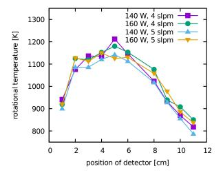
Figure 4. Rotational temperature profile along the discharge axis with aerosol for different power and working gas flow rate.
