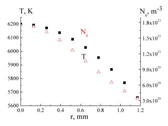
Figure 1. Radial distributions of plasma temperature and electron density of arc discharge between composite Cu-Cr electrodes at current 3.5 A.
