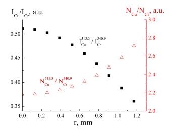
Figure 2. The ratio of the radiation intensity of the spectral lines Cu I 515.3 nm and Cr I 540.9 nm ( $\blacksquare$ ). The ratio of concentrations of copper and chromium atoms ( $\triangle$ ).
