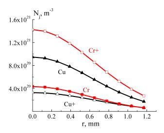
Figure 4. The radial distributions of Cu, Cr atoms and  $Cu^+, Cr^+$  ions concentrations.
