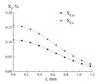
Figure 3. The radial distributions of copper and chromium vapours contents in plasma of electric arc discharge between composite Cu-Cr electrodes at current 3.5 A.
